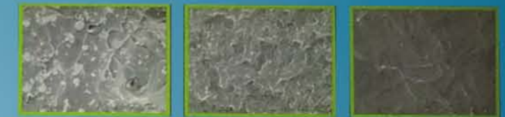
Gravity Cast (1 Bar) Low Pressure (10 Bar) Cast in Hadi (120 Bar)
